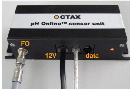
Fig. 4: Connection of the grey fiber optic (FO) to pH Online™ outside the incubator. Data connection to OCTAX Log & Guard™ via serial cable (silver cable; data). Power supply is plugged in the 12V DC port (black cable).
