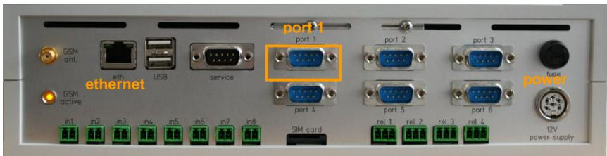
Fig. 5: Backside of the OCTAX Log & Guard™ device with highlighted ports for Ethernet, RS 232 data connection and 12V DC power supply.
