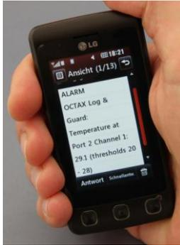
Fig. 21: Mobile phone display showing a temperature alarm message sent by OCTAX Log & Guard™
