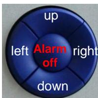
Fig. 7: Control keys of OCTAX Log & Guard™.
